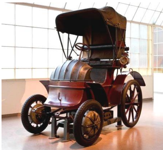
“Lohner-Porsche” Pure electric vehicle Front wheel drive
