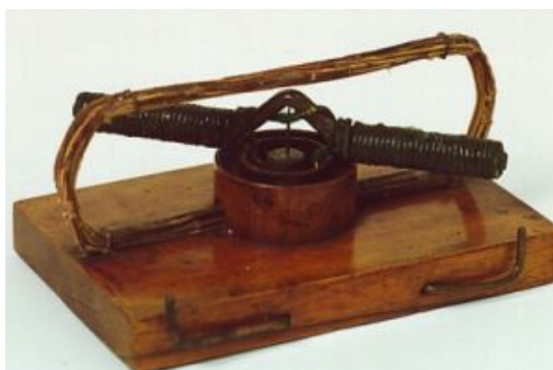
Jacobi's first electro-motor
