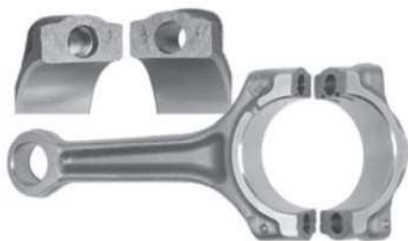
Figure 4.6: Fracture surfaces of the big end bore, manufactured by cracking
